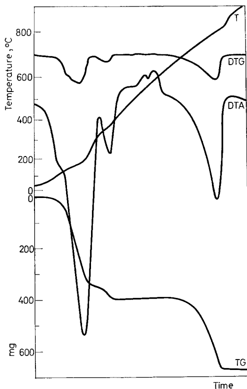
Fig. 2. Thermoanalytical curves of \text{FeSO}_4 \cdot 7 \text{H}_2\text{O} using multiple sampleholders
